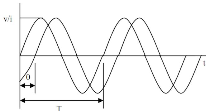
**Figure 2. Two sinusoidal waves with phase difference**
