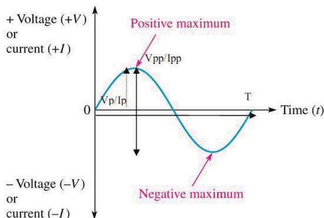
Fig 1: Graph of one cycle of a sine wave
