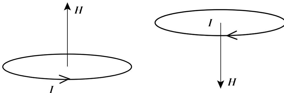
The magnetic field of a current-carrying conductor can be further concentrated by forming multiple turn loops (coils). This, in effect, increases the magnetic field by a multiplication factor equal to the number of turns  $N$ .
