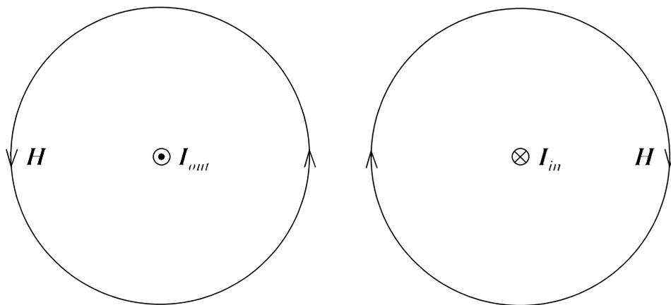
The magnetic field of a current-carrying conductor can be concentrated by forming the conductor in the shape of a loop. The magnetic field direction through the loop can also be determined by the right hand rule. Aligning one's fingers in the direction of the loop current, the thumb defines the direction of the magnetic field through the loop.
