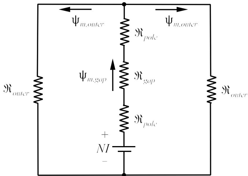
The reluctance components for the magnetic circuit are
