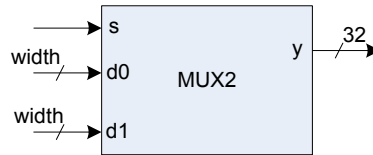
Figure 3: Entity of the 2x1 Multiplexer
