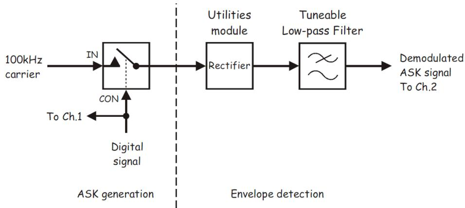
Figure 7: an ASK generation and demodulation
