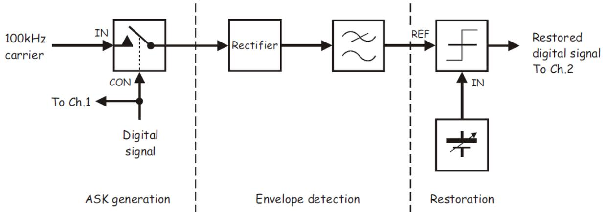
Figure 9: an ASK generation, demodulation, and digital signal restoration
