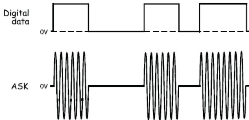
Figure 1: an ASK signal (below) and the message (above)
